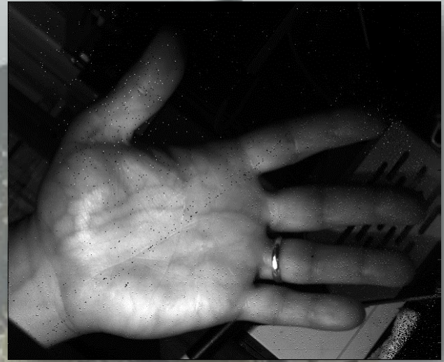
5ms exposure, FPA InGaAs Cooled, LED at 940nm in front of the hand
