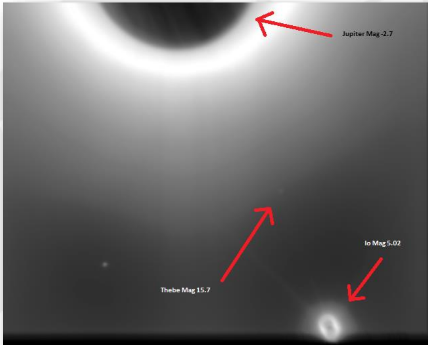
Filter J, Jupiter in Linear (CTIA) response stack of 40 exposure of 5s each with NDRO readout noise reduction
