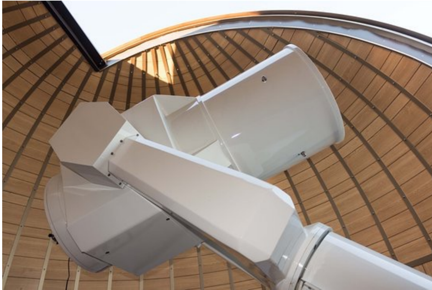
Optical telescope Richey-Chrétien 50 cm primary mirror
