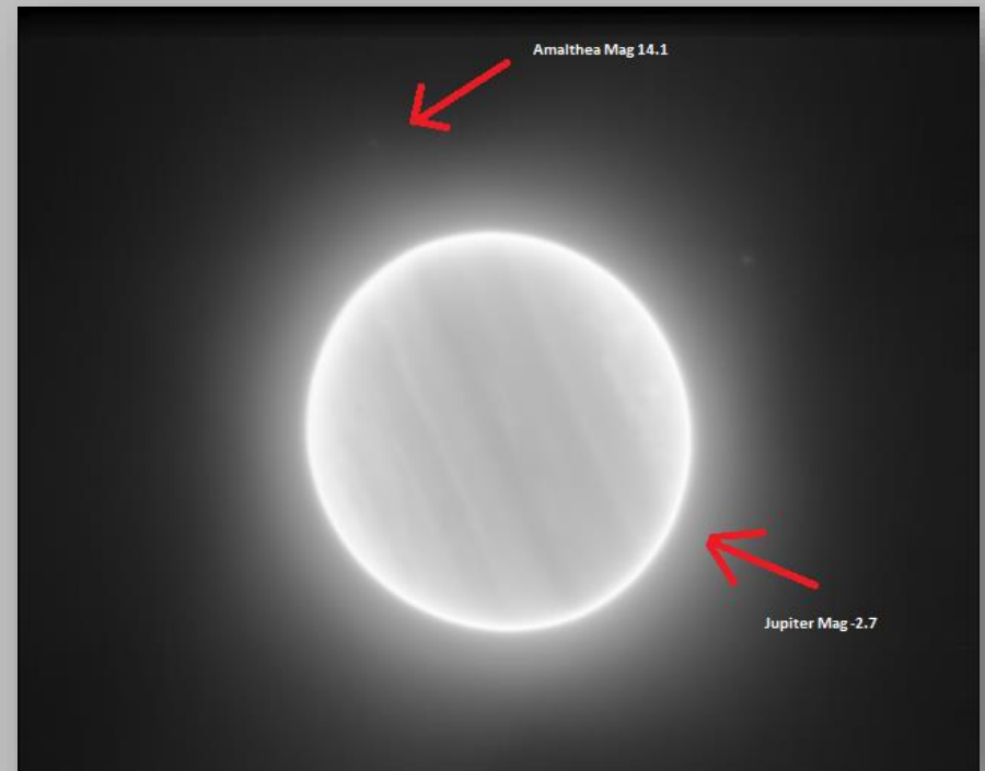
Filter J, Jupiter in Linear-Log response stack of 80 exposure of 2s each with NDRO readout noise reduction
