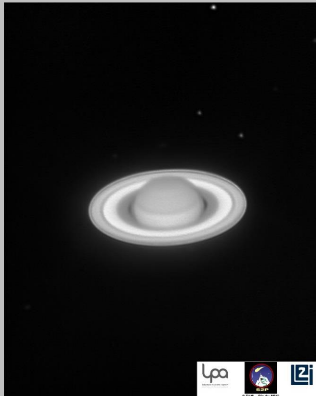
Filter J, Stack of 40 exposures of 10s. (Log and Lin response mixed on each) 11/07 22H55 UT
