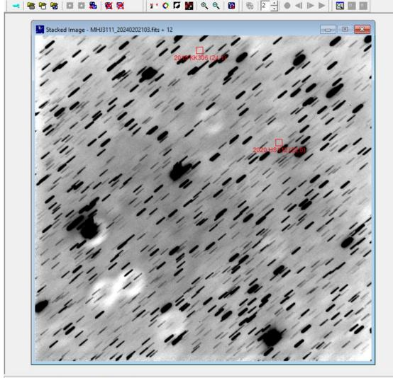
Astrometrica implements the stack and track technique. The target's movement needs to be known in advance.
