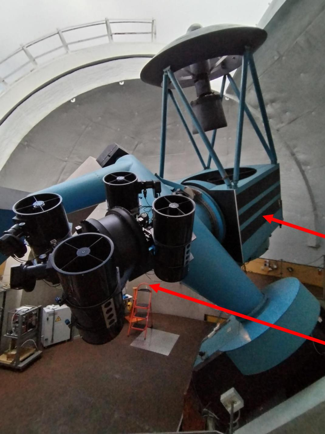
The “Gian Domenico Cassini” is a 1.5-m F/4.8 Ritchey-Chretien telescope with a CCD plate scale of about 0.6 arcsec/pixel and a field of view of 13 x 13 arcmin. “Cassini” is Italy's second-largest optical telescope.
