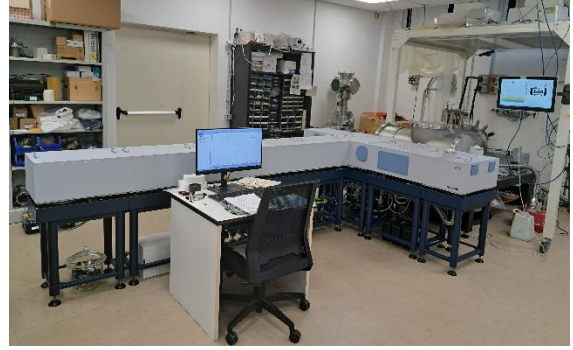
Figure 1: Experimental setup, consisting of a Fourier Spectrometer coupled with a simulation chamber (in grey behind the FTIR)
