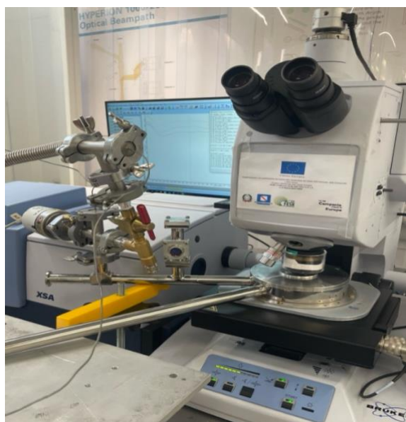
Figure 1: Experimental setup composed of a cryogenic cell that allows a controlled environment for the sample, and a microscope coupled with an FTIR spectrometer that enables the acquisition of the spectral radiance of the samples.
